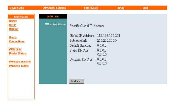
Basic status can be "Specify Global IP Address," "Obtain Global IP Address Automatically (DHCP)," or "PPP over Ethernet (PPPoE)," depending on which of these is currently selected in the Basic Setup menu's Broadband Router settings panel.
